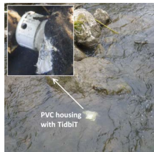
FIGURE 7. PVC HOUSING EPOXIED TO A ROCK.
